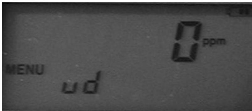
"Oppm ud (ud=under)" will display leaks in steps. The steps are 0ppm, ud 500ppm, ud 1000ppm, ud 3000ppm, ud 5000ppm, ud 9999ppm
