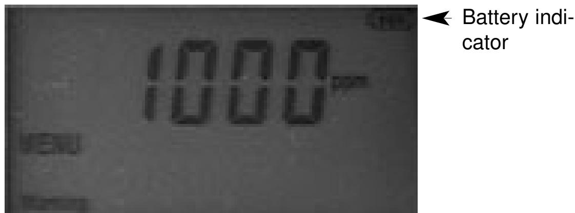
The battery indicator will show full capacity ( ), half capacity ( ), one quarter capacity ( ), and replace ( ).
