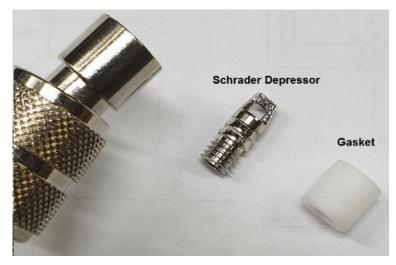
3 Install the gasket and screw in the Schrader depressor. (New Schrader depressor and gasket are part number A670)
